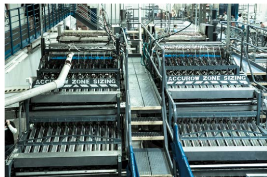
The Accurow cherry sizer was the first machine Stemilt had that sized cherries with an automated system.
